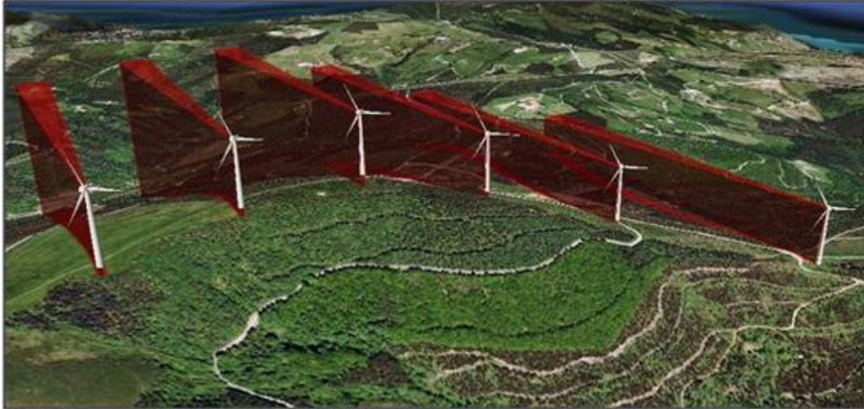
Figure 4.13.1. Example of calculations for a WTG-generated zone where a radar beam is blocked 132
